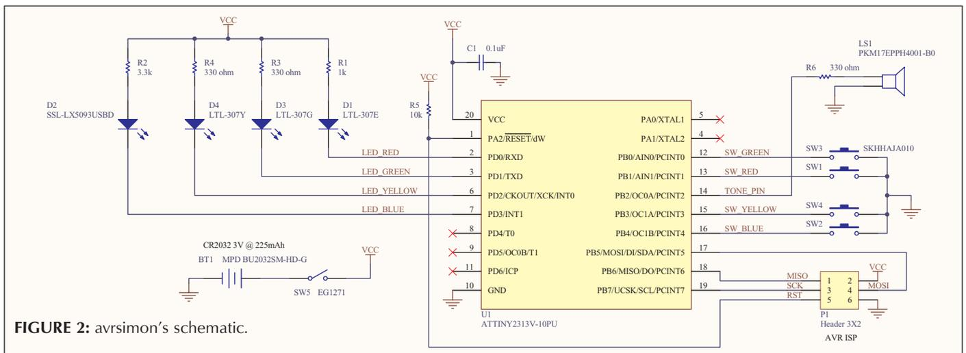
**FIGURE 2:** avrsimon's schematic.
