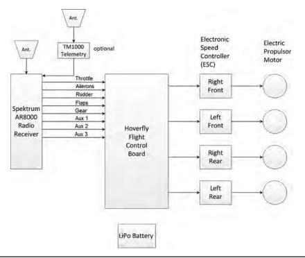
FIGURE **1.8** Main electrical/electronic Elev-8 components.
