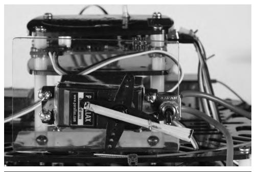
FIGURE 1.13 Servo-control kill switch.
