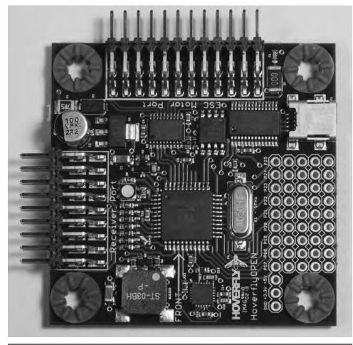
FIGURE 1.7 HoverflyOPEN controller board.
