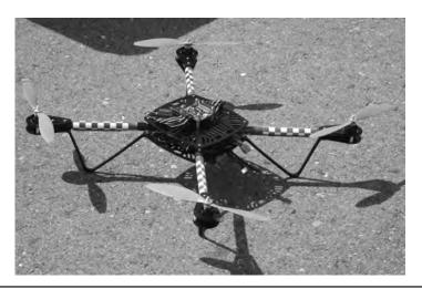
FIGURE 1.9 Basic Elev-8 quadcopter.
