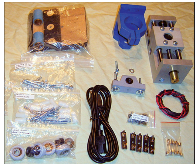
■ FIGURE 9. Starting at top center and going clockwise: table supports, tool holder, Z axis assembly, hookup wire, fuses, fuse holders, power cord, lead screw bearings and clamps, and assorted bags of hardware.
