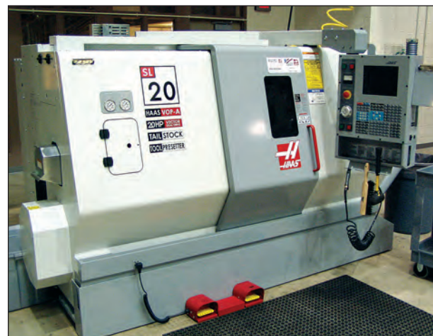
■ FIGURE 2. A CNC turning center in the FAME Lab in the Leonhard Building at Penn State. (c) 2005 Nathaniel C. Sheetz.
