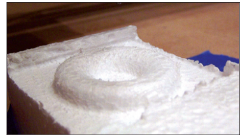
■ FIGURE 19. First cut of Torus (rough lower edge due to mismatch of cutter and Z depth).
