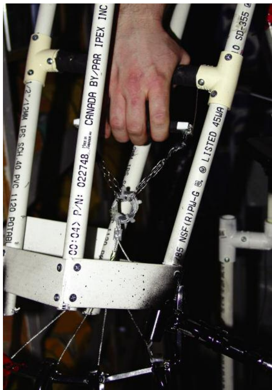
FIGURE 19. Pulling the bar would make the hand open and close.
