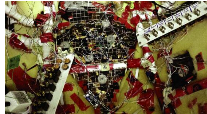
FIGURE 21. The back of the chest gears, and all the system emergency shutdown switches (before the Solarbotics upgrade).
