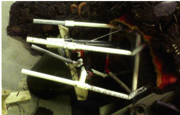
FIGURE 11 The interior of the weapon arm, with the drill mounted and made accessible to the operator.
