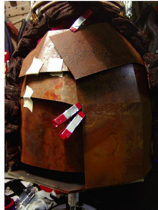
FIGURE 14. Shaping the face out of some scraps of sheet metal I had laying around.
