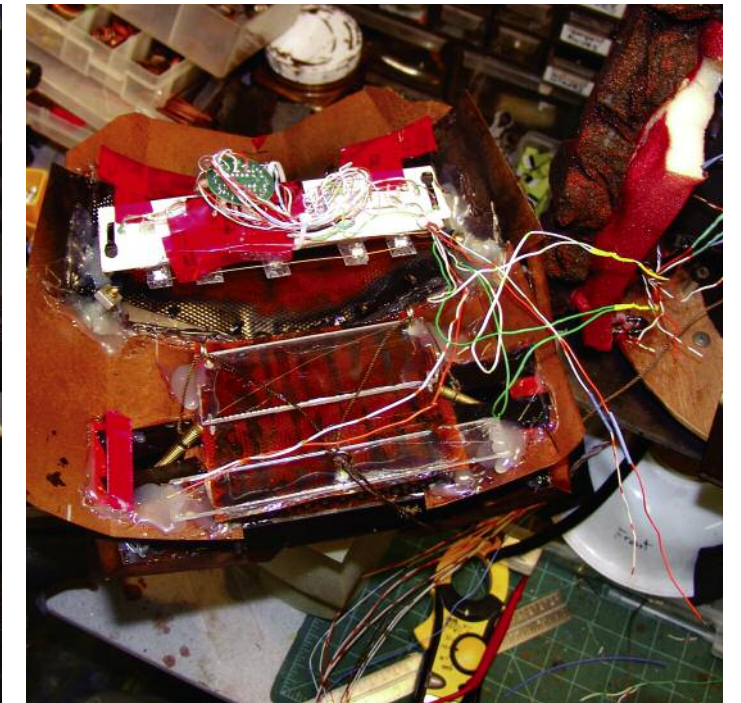
FIGURE 15. The electronics of the face, and the pulley system that activates the jaw.
