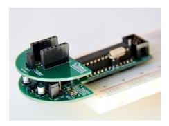
**Important:** If the module is inserted back-to-front, and power applied to the parent board, both the module and the parent Toadstool prototyping board could be irreparably damaged.
