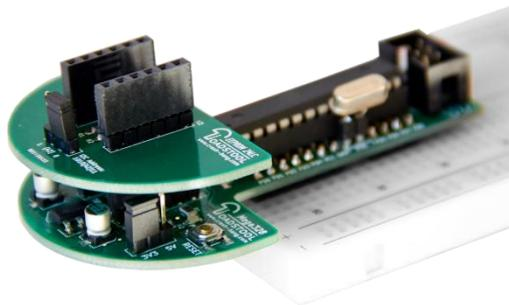
The Toadstool *Mega328* is a prototyping board – it houses a microcontroller and plugs directly into a breadboard. There are a number of other Toadstool boards containing a range of microcontrollers from various manufacturers. All these boards come with a standard header interface that allows standardised breakout boards to be connected.
