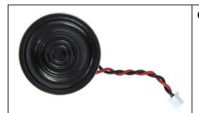
Cut the connector off the end of the speaker pigtail
