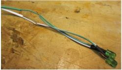
Twist together the two white leads from the two LEDs with the white lead from the pig tail. Do the same for the other color lead as shown.
