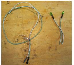
Cut the two LEDs off from the end of the two pigtails. Keep one of the pigtails and set the other one aside.
