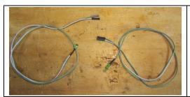
The two unmodified LED pigtails. *Note: the wire color and LED color may vary from kit to kit.*
