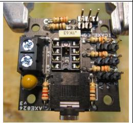
Insert the power connection screw terminals, and the servo headers and solder them into place.
