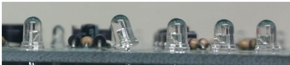
Figure 30 - LED not snug against board, needs rework
