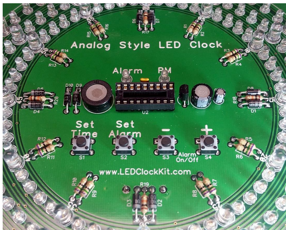
Figure 38 – Check the orientation of the parts
