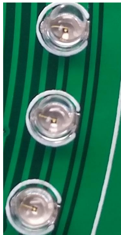
Figure 22 – Internal wires point the same way
