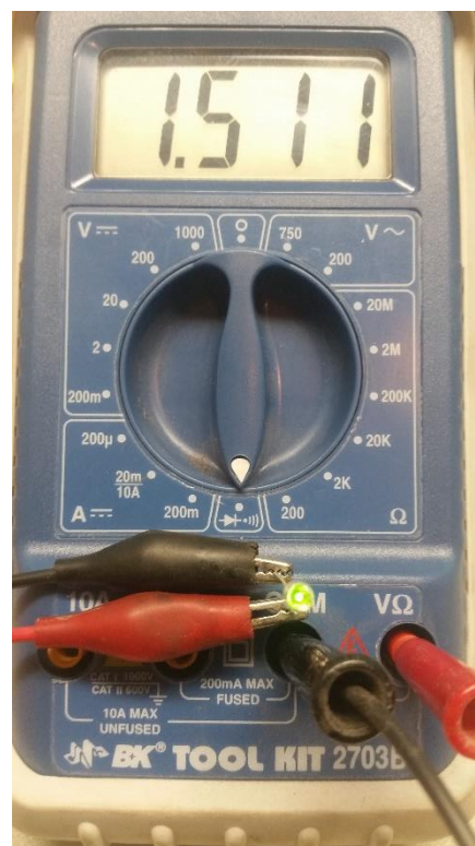
Figure 20 Using a meter to light an LED
