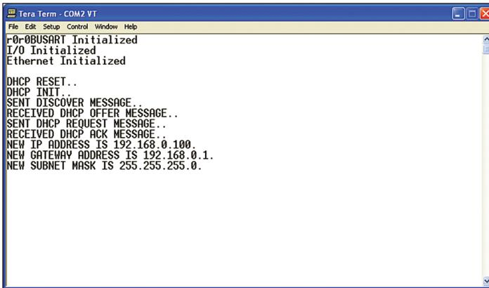
■ **SCREENSHOT 1.** This all goes back to my love of using an embedded device's RS-232 port as a debugging tool. During the debugging phase, if I didn't get the message I wanted to see here, or the messages were looping, I would then turn my attention to reading dumps and registers produced by the Microchip REAL ICE to find a fix.
