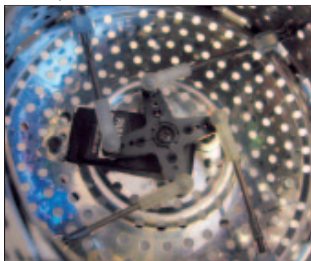
■ FIGURE 15. Move the servo through its length of travel, then insert the center screw to hold the servo horn in the position that allows the flower to go from open to closed.
